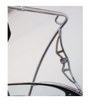
The rear switch blades can now be installed by attaching the top switch blade fitting to the fitting located on the upper section of the front leg. The clamp located on the base of the switch blade will be connected to the lower side rail. We recommend making sure that the clamps on both sides of the tower are located the same distance from the end of the side rail so that your tower looks symmetrical.
