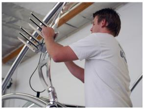
To install the board rack fingers, use the socket head cap screws provided and attach the fingers to the diamond shaped plate. This diamond plate will then be installed to the rear switch blade legs.
