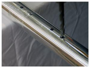
Following the pilot holes you just drilled, use a 27/64" drill bit to create the clearance hole for the joining bolts. As each hole is drilled we recommend inserting each bolt so that it keeps the parts aligned while drilling the next hole.
