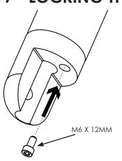
Once you are happy with your tower installation and all of the fittings are lined up to allow the tower to fold and function correctly it will then be important to firmly lock the fittings in place to prevent any unwanted rotation or loosening. We recommend using threadlocker during this step.
