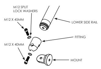
The mounting feet will need to be assembled to the side rail fittings, followed by attaching them to the side rails.
