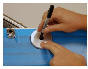
Once the desired position is achieved, place one of the nylon mount washers over the piece of tape and trace around it with a permanent marker.
