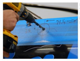
If necessary, you should move the wires out of the way while you drill. We recommend drilling a small pilot hole which will keep the 17/32" drill bit from walking (moving). A small rat tail file can be used to ease the edge and keep the gel coat from chipping. Be careful of wires!
