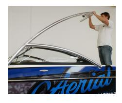
Insert the front leg hinge joint into the lower section of the front arm (repeat for the other side). Its important not to completely tighten the fittings as some adjustment will necessary before the installation is complete.
