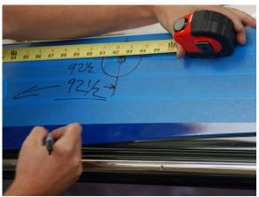
It is best to take measurements from the back of the boat and mark with blue tape. Be sure to measure from the same point on both sides.
