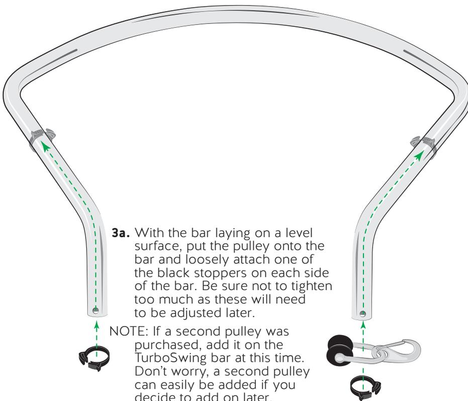
3a. With the bar laying on a level surface, put the pulley onto the bar and loosely attach one of the black stoppers on each side of the bar. Be sure not to tighten too much as these will need to be adjusted later.
