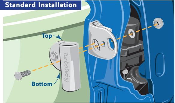
2a. Piece together the M8 x 25 bolt with the grooved locking nut onto the TurboSwing tube holder.
