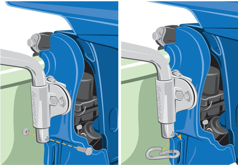
4. Complete your TurboSwing install by inserting the supplied carabiners into the holes at the bottom of the TurboSwing tube. If you are looking for a more permanent installation, feel free to replace the carabiner on either side with the supplied M8x45 bolts and M8 Lock Nuts.
