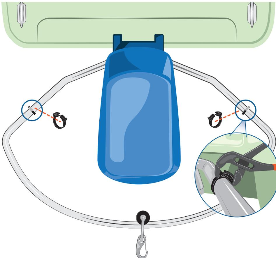
3j. Tighten existing stopper **on one side** and add one additional stopper next to it.
