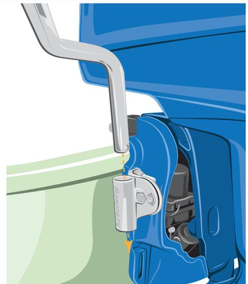
**!** 3b. Trim motor up to allow room for the bar to be inserted into the tube holders.
