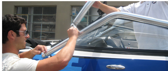
IMAGE SHOWS THE SIDE SECTION BEING ATTACHED TO THE SIDE RAIL.
